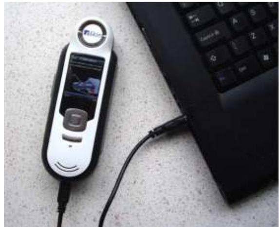
**Note:** Some computers have low power USB ports which are typically located at the front. It is recommended that the e-Skin device is ONLY connected to high power ports.
