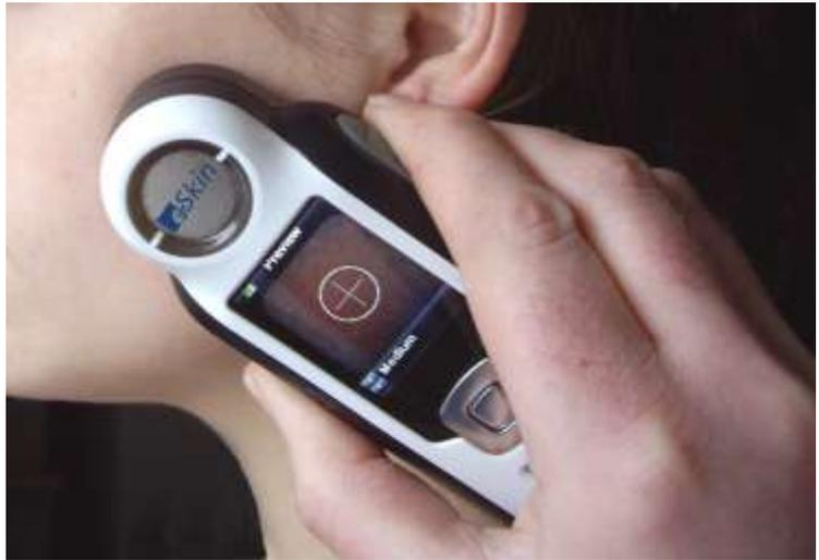
An audible "camera-click" sound indicates the start of the measurement. A progress bar appears at the bottom of the display to indicate the measurement status. Colour information appears in the display after the progress bar reaches 100%.
